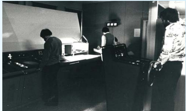
Shipbridge simulator with steering stand but no outside view
